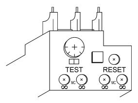
Figure 14. Over Current Relay
